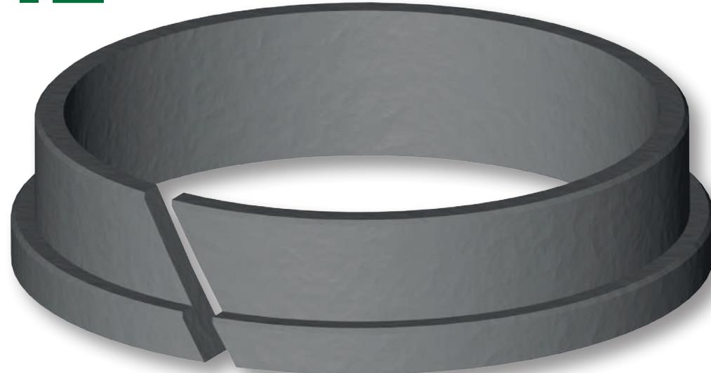
The Aston Seals FIL type guide rings have been developed to substitute traditional bronze guides in hydraulic cylinders. They guide the rod and prevent metallic contact with the cylinder head when radial forces act perpendicular to the direction of movement. Chamfered edges prevent splintering of the material during assembly and make the installation into the groove easier.
