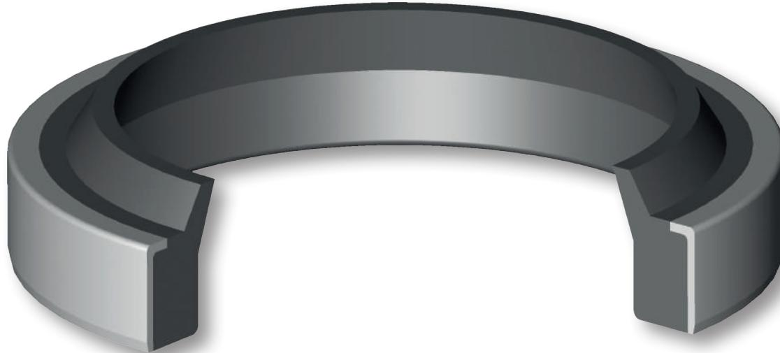
The function of the Aston Seals SMA wiper ring is to prevent introduction of dust, dirt and foreign matter into the system. This is achieved by a special wiper lip which produces a very effective cleaning action, prevents the development of scores, protects the guiding parts and extends the service life of the axial moving rod seals.
