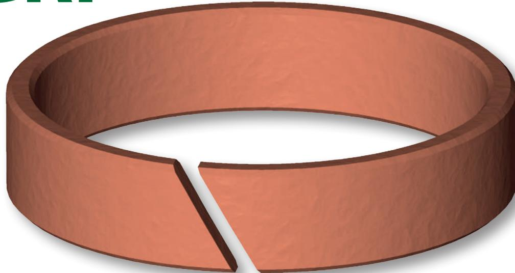
The Aston Seals GRF type guide rings have been developed to substitute traditional bronze guides in hydraulic cylinders. They guide the rod or the piston and prevent metallic contact with the cylinder when radial forces act perpendicular to the direction of movement.
