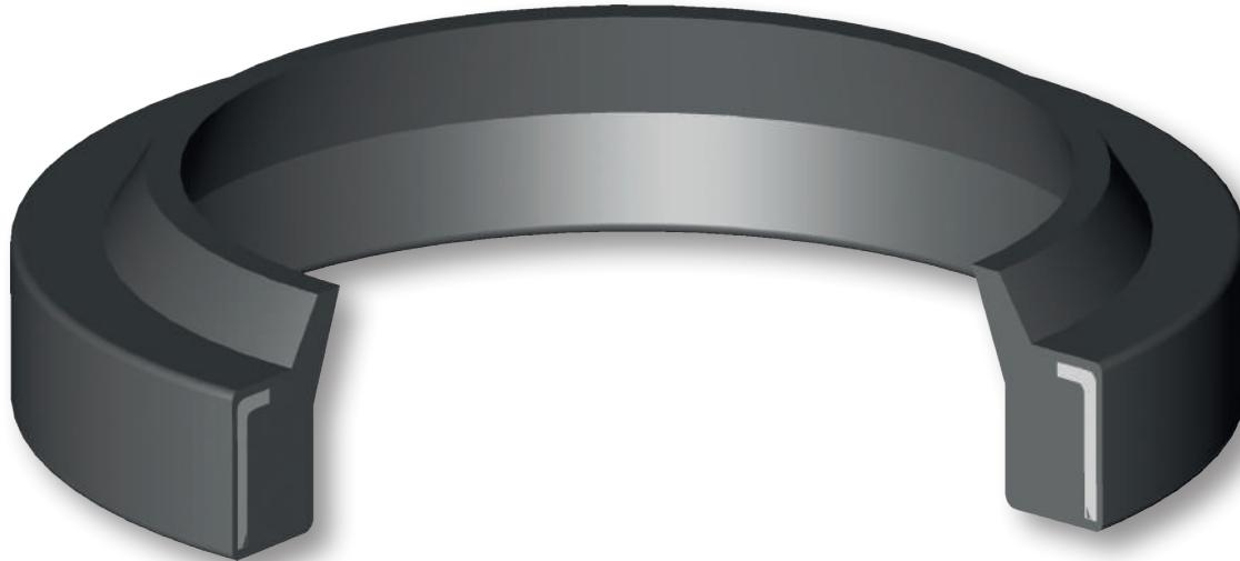
The function of the Aston Seals SMI wiper ring is to prevent introduction of dust, dirt and foreign matter into the system. This is achieved by a special wiper lip which produces a very effective cleaning action, prevents the development of scores, protects the guiding parts and extends the service life of the axial moving rod seals.
