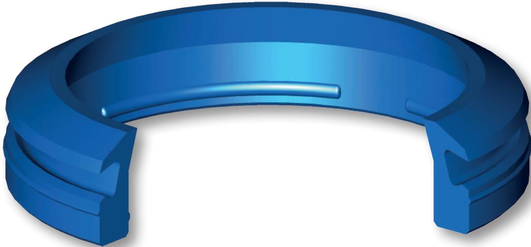
The function of the Aston Seals SAC wiper ring is to prevent introduction of dust, dirt and foreign matter into the system, to protect the guiding parts and to extend the service life of the axial moving rod seals.
