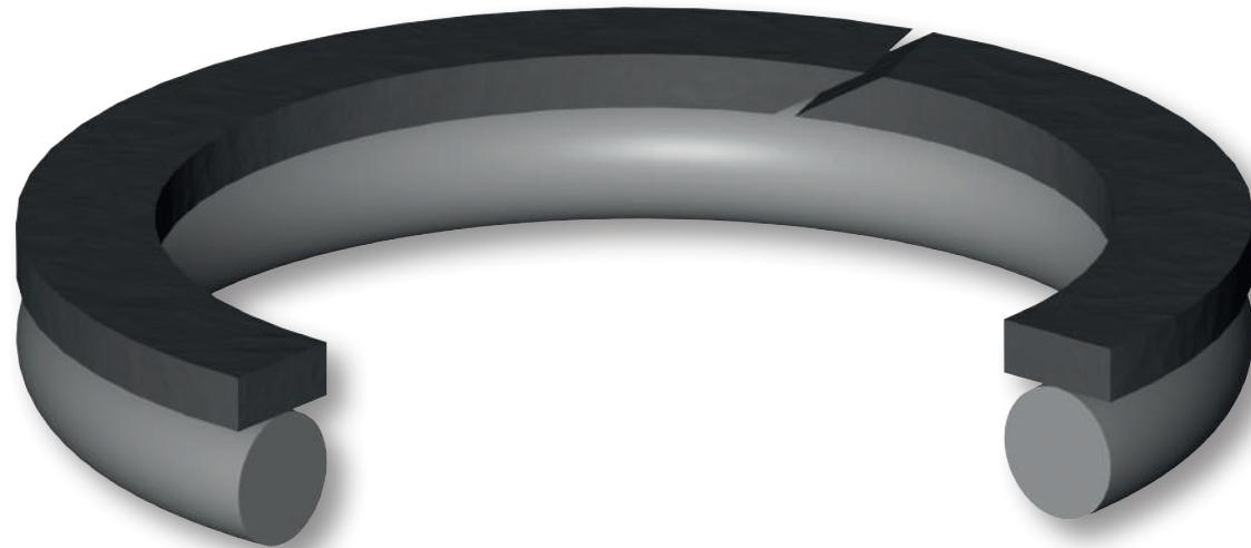
The function of ring type Aston Seals BRT is to avoid the extrusion and damage of the O-Ring that normally occurs in the presence of large gaps or high pressure.
