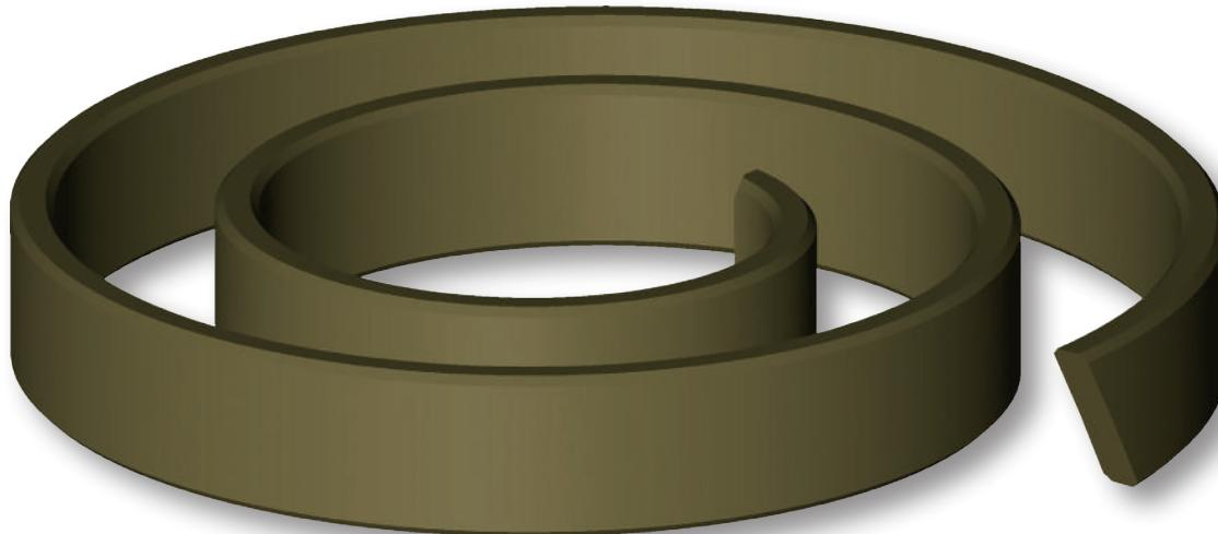
The Aston Seals MRB type guide rings have been developed to substitute traditional bronze guides in hydraulic cylinders. They guide the rod or the piston and prevent metallic contact with the cylinder when radial forces act perpendicular to the direction of movement.
