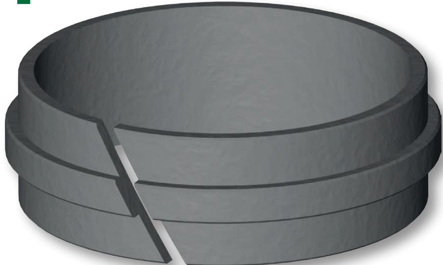
The Aston Seals FIT type guide rings have been developed to substitute traditional bronze guides in hydraulic cylinders. They guide the rod and prevent metallic contact with the cylinder head when radial forces act perpendicular to the direction of movement.
