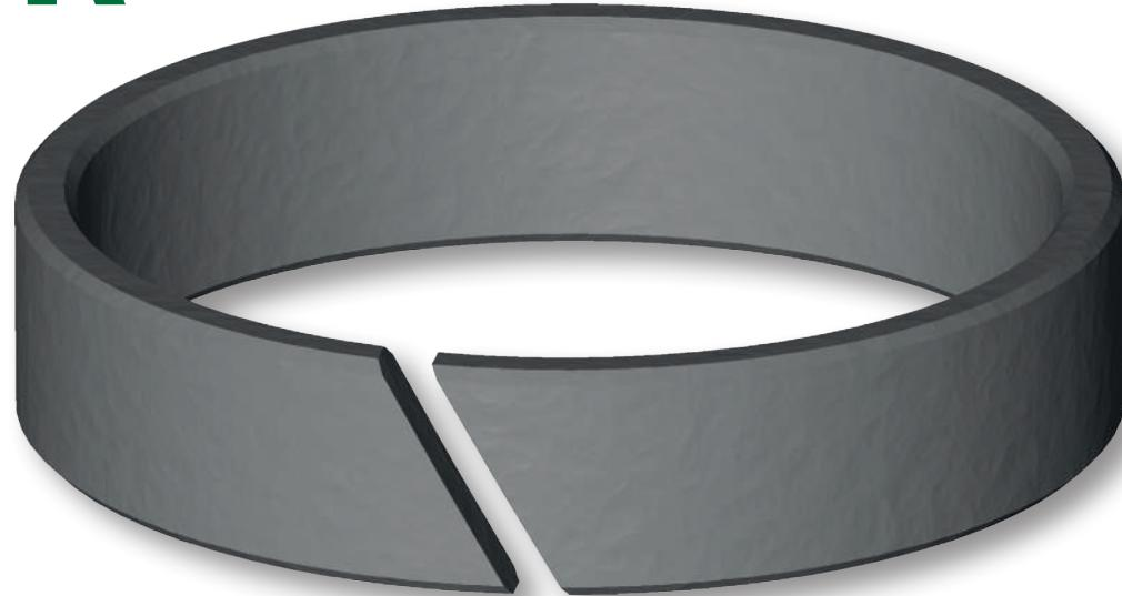
The Aston Seals FR type guide rings have been developed to substitute traditional bronze guides in hydraulic cylinders. They guide the rod or the piston and prevent metallic contact with the cylinder when radial forces act perpendicular to the direction of movement.
