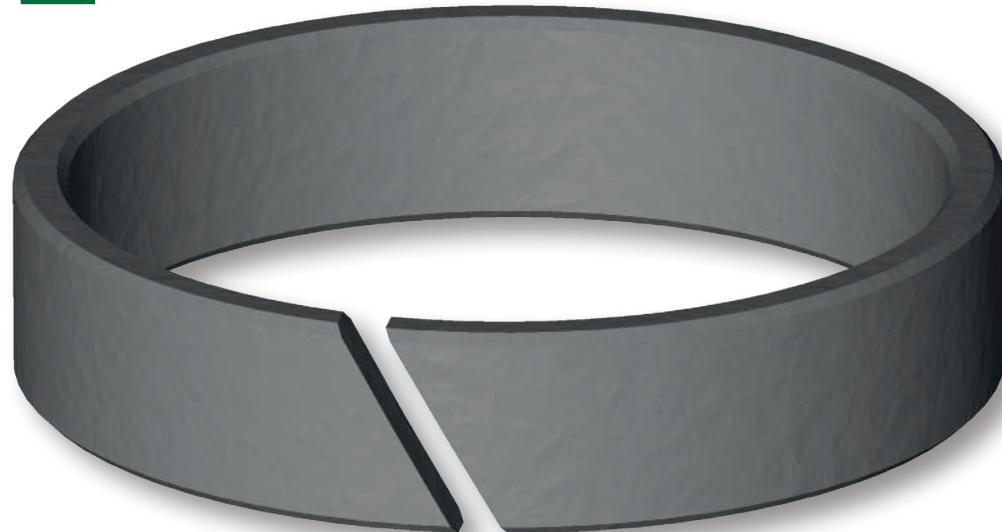
The Aston Seals FE type guide rings have been developed to substitute traditional bronze guides in hydraulic cylinders. They guide the piston and prevent metallic contact with the cylinder when radial forces act perpendicular to the direction of movement.
