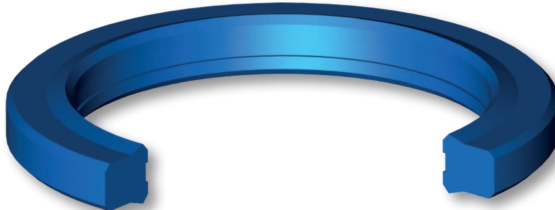
The polyurethane seal type Aston Seals PFS has been developed to assure a SAE flange sealing and to substitute traditional O-Rings when they are not suitable due to difficult conditions such as high pressure or rough surface finish.
