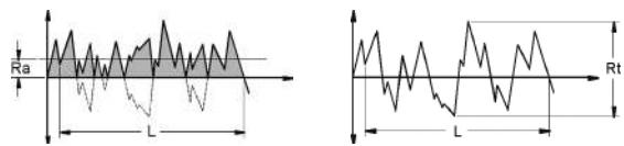
The standard method of measuring roughness is by an average value of the profile variation from a centre line over a reference length (L). This is known as Centre Line Average (CLA), now commonly expressed as Ra ( $\mu\text{m}$ ).
