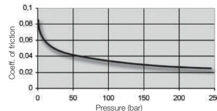
The dry friction of typical seal materials rubbing on a smooth, dry seal surface may be anything from  $\mu=0.4\div 1$ . For lubricated surfaces the range is much lower, for example,  $\mu=0.02\div 0.10$ . This is particularly true in the case of elastomers. Fabric materials and impregnated fabrics show similar values of " $\mu$ " but usually with less variation, for example  $\mu=0.04\div 0.08$  for lubricated conditions.
