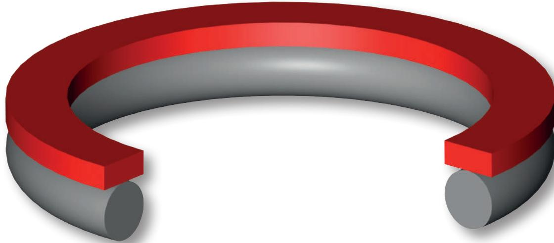
The function of ring type Aston Seals AM is to avoid the extrusion and damage of the O-Ring that normally occurs in the presence of large gaps or high pressure.
