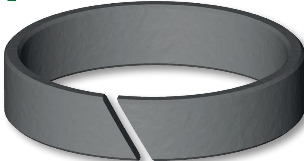
The Aston Seals FI type guide rings have been developed to substitute traditional bronze guides in hydraulic cylinders. They guide the rod and prevent metallic contact with the cylinder head when radial forces act perpendicular to the direction of movement. Chamfered edges prevent splintering of the material during assembly and make the installation into the groove easier.
