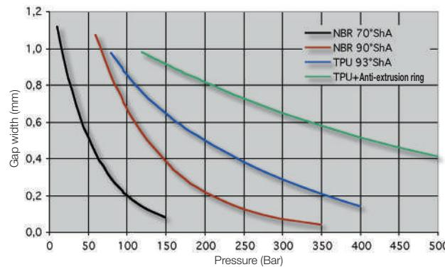
When calculating the gap widths, the given play at the guide (fitting tolerance) and the elastic stretching of the cylinder bore under pressure must be considered. Otherwise the permissible gap width will be exceeded with offset installation of the rod or piston. If the permissible gap widths are exceeded, then extrusion wear (see figure) occurs at the back of the seal and this destroys the seal after a short period of time.
