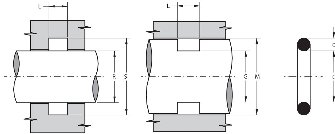
Other sizes not present in the above table can be provided, depending on the O-Ring chord "c", in according to the following scheme:
