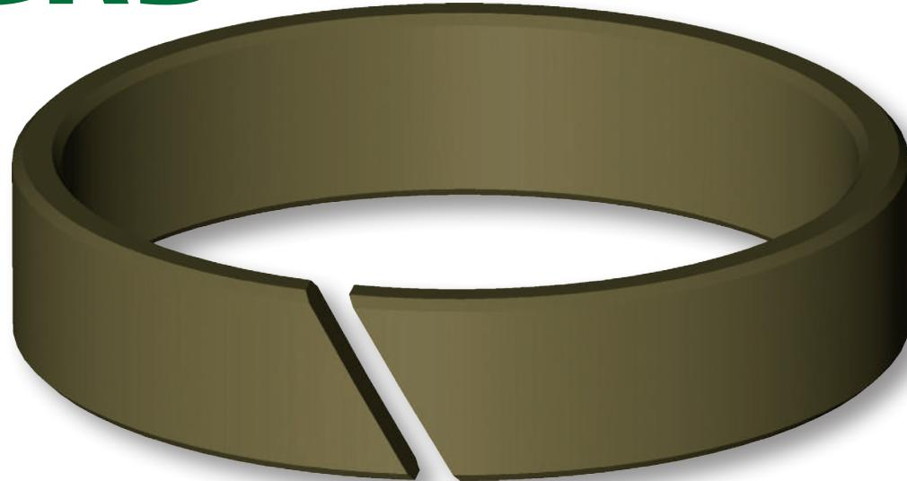
The Aston Seals GRB type guide rings have been developed to substitute traditional bronze guides in hydraulic cylinders. They guide the rod or the piston and prevent metallic contact with the cylinder when radial forces act perpendicular to the direction of movement.
