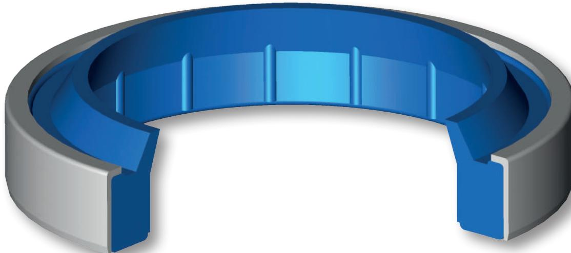
The function of the Aston Seals SAF/GM wiper ring is to prevent introduction of dust, dirt and foreign matter into the system. This is achieved by a special wiper lip which produces a very effective cleaning action, prevents the development of scores, protects the guiding parts and extends the service life of the axial moving rod seals.
