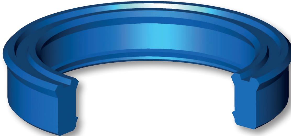
Wear and dry run are largely prevented by additional lubricant retained within the gap created by the secondary lip. In some cases this second sealing lip may even act as a substitute for a costly tandem sealing system when complete sealing under certain working conditions can only be achieved by two seals placed one behind the other in separate housing.
